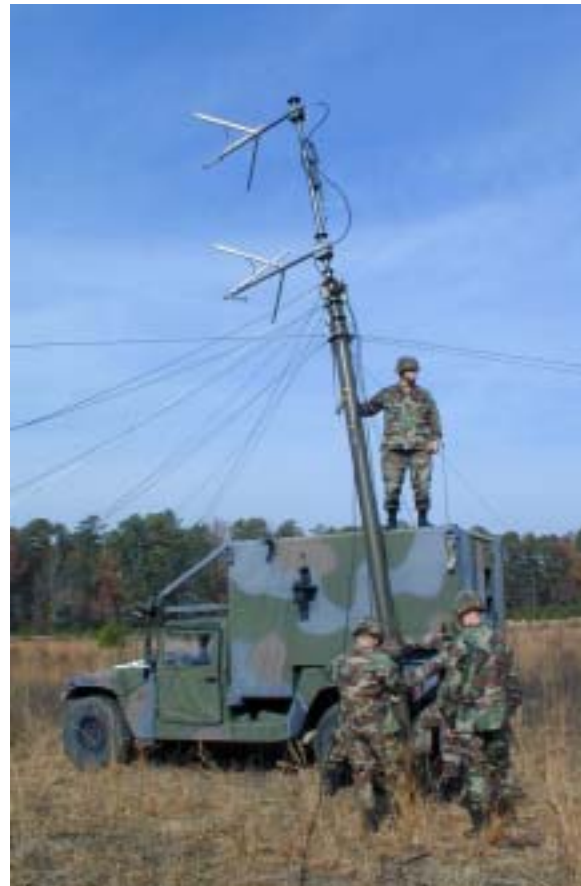
Soldiers erect the antenna of the Special Operations Media System-Broadcast (SOMS-B) capable of providing local radio and television support including editing of radio and audiovisual products.
